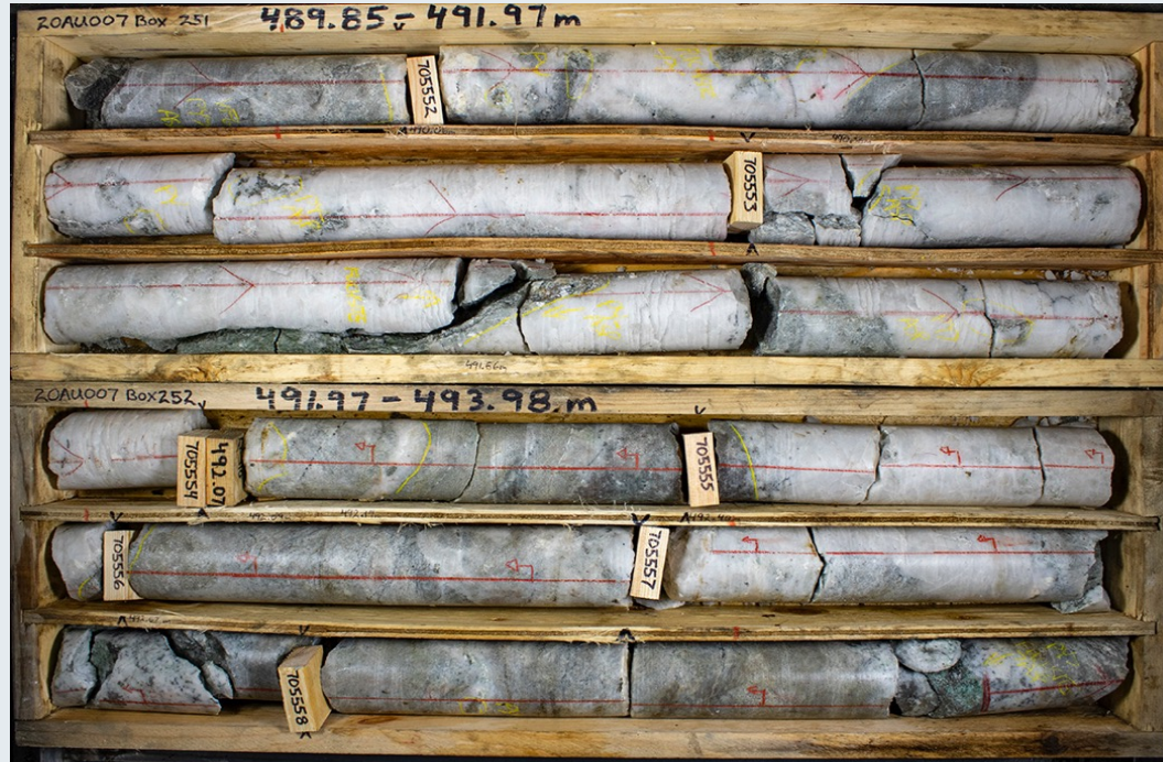
Hole#7 (20AU07) Quartz vein with fuchsite and sulphides - arsenopyrite, pyrite, pyrrhotite (did not carry Au grade)
