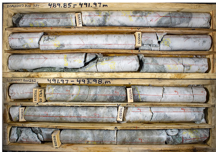
Figure 4 Drill core from 2020 hole#7 (20AU07) 7m thick Quartz vein from 488m with fuchsite and sulphides – arsenopyrite, pyrite, pyrrhotite; part of broader 22m zone of quartz veins. Currently the subject of near-miss analysis using fluid inclusion analysis.
