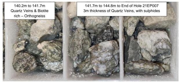
Figure 1 Typical Quartz Veins and sulphides in Hole ID 21EP007: 4.6m interval from 140.2m to 144.8m (end of hole).
