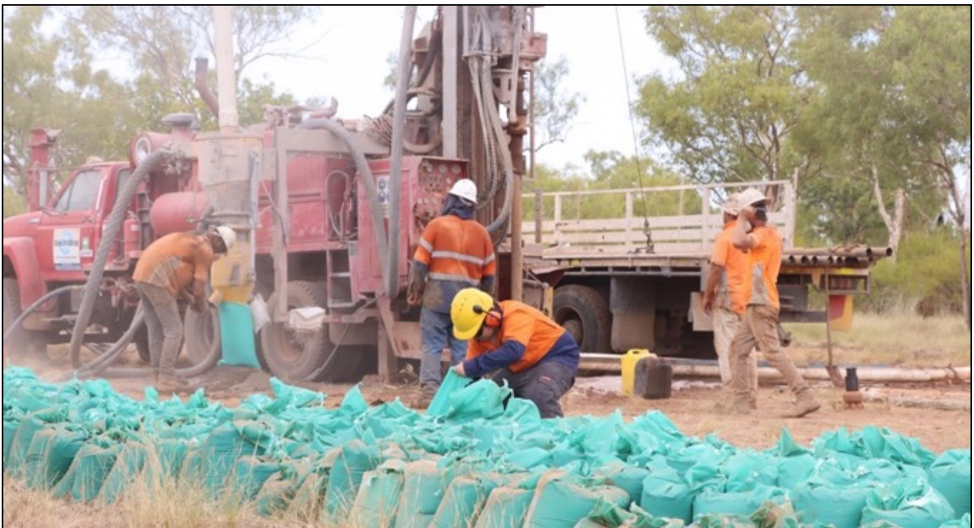
Figure 14 Drilling (RC rig) on the Benmara Project October 2021. RML staff member (Henry) pictured taking spot samples for geological logging from green bag of drill cuttings. (RC = Reverse Circulating style of drilling)
