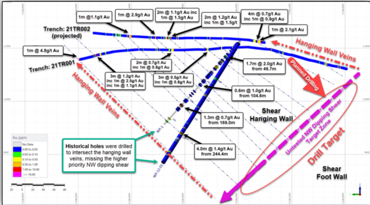
Figure 6 Tourmaline Ridge Prospect cross section including full assay results on trench 21TR001 and 21TR002. Historical holes WP12-01 and WP-1 are included, aiding interpretation of antithetic hanging wall veins relative to an interpreted northwest dipping shear.
