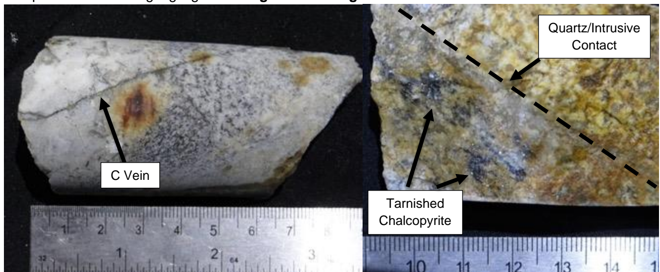
Figure 10 Elaine Prospect, HoleID 00ED-02, 69.7m, (left) mm pyrite-chalcopyrite vein cross cutting coarse intrusive/quartz vein contact (C Vein) and (right) zoom in on tarnished chalcopyrite within quartz vein (B Vein).
