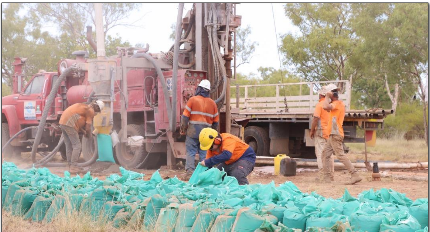
Figure 15 Drilling (RC rig) on the Benmara Project October 2021. RML staff member pictured taking spot samples for geological logging from green bag of drill cuttings. (RC = Reverse Circulating style of drilling)
