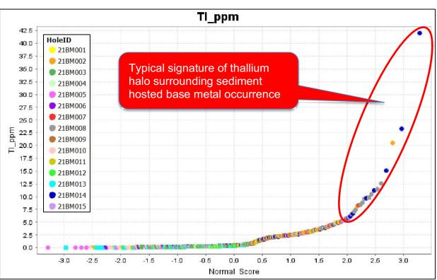
Figure 5 Thallium (TI) results coloured by RC drillhole. Note holes 21BM001, 21BM002, 21BM007, 21BM008, 21BM014 and 21BM015 intersected thick carbonaceous siltstone and shale units.
