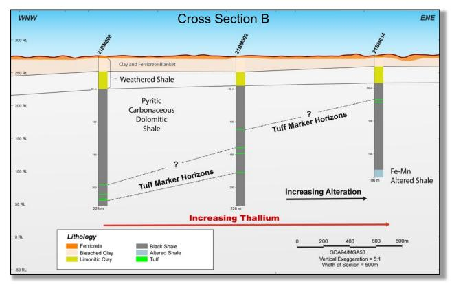
*Figure 8 Cross Section B – with increasing thallium trace element to the east indicating a vector towards mineralisation*
