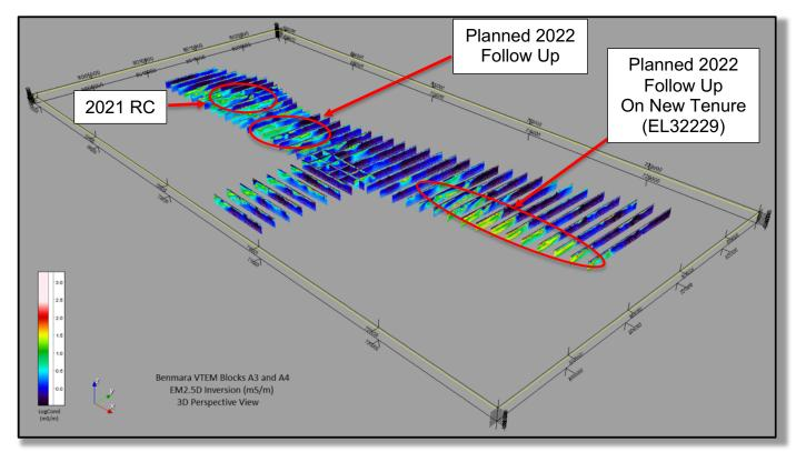
Figure 9 - 3D perspective view looking north-west on the Benmara 2.5D Inversion. 2021 RC location relative to planned 2022 drilling areas
