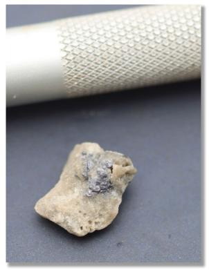
Figure 3 Galena (lead sulfide) HoleID: 21BM006 from 166-167m (depth)
