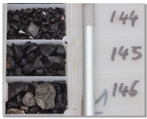
Figure 2 Typical pyritic shale HoleID: 21BM001 from 144-146m (depth)
