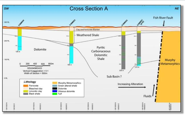
Figure 7 Cross Section A
