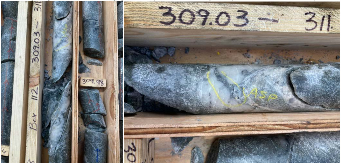
Figure 9 Example of a quartz-sulphide vein “dilation zone” intersected in hole 20AU08. The photo on the left is an interval of NQ drill core from 309.18 - 309.78m. The photo on the right is a zoom in on the interval 309.18 - 309.38m with an arsenopyrite vein cross cutting a quartz vein highlighted with yellow markings.
