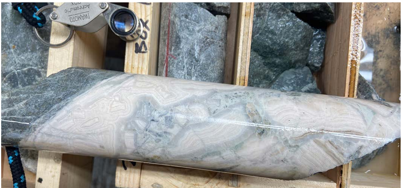
Figure 10 drill core (HQ) interval 212.35 – 212.50m hole 20AU09. Example of a brecciated colloform quartz vein “dilation zone”.
