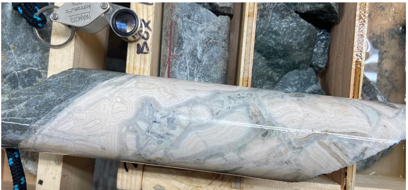
Figure 12 drill core (HQ) interval 212.35 – 212.50m hole 20AU09. Example of a brecciated colloform quartz vein “dilational zone”.
