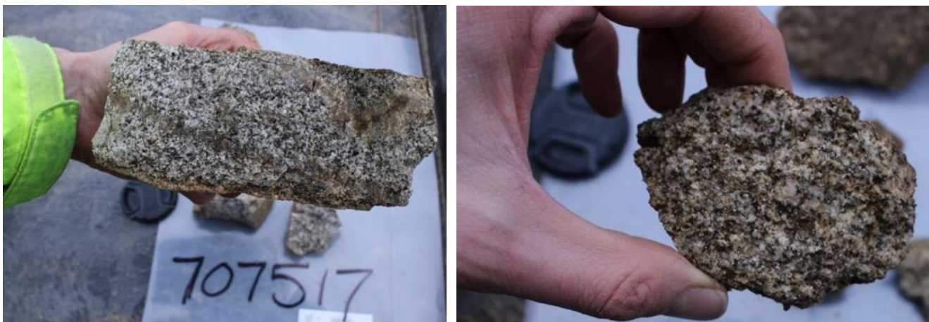
Figure 5 Quartz-feldspar-biotite granite samples from road cut 20AT001T. Sample 707517 (left) assay returned 1.63g/t Au from 66-67m and includes 1-6mm wide quartz veins (sheeted vein sets). Sample 707529 (right) assay returned 1.89g/t Au 78-79m.
