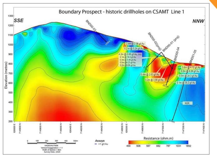
Figure 6 Historic drilling overlaying Line 1, 2D CSAMT section, looking west. Gold intersections coincide with a shallow CSAMT anomaly. Deeper anomaly remains untested. Boundary Prospect, Northern Zone, East Pogo Block, 64North Project Alaska.
