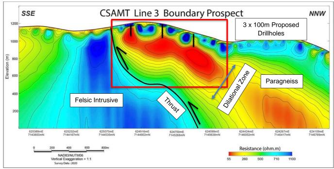
Figure 5 Example of reconnaissance drillhole design on Line 3, 2D CSAMT section looking west, within the Central Zone, East Pogo Block, 64North Project Alaska. Shallow Line 3 anomaly is located 2.5km southwest of historic high grade gold intersections.
