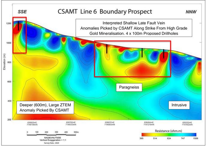
Figure 3 Example of reconnaissance drillhole design on Line 6, 2D CSAMT section looking west, within the Northern Zone, East Pogo Block, 64North Project Alaska. Shallow line 6 anomalies are located 500m east of historic high grade gold intersections.
