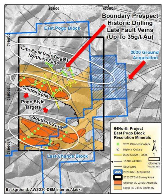
Figure 2 East Pogo Block: Planned shallow reconnaissance ridge line drilling collar locations. Central and southern holes targeting pogo-style mineralisation interpreted as dilation zones along thrust contact. Northern holes targeting late fault veins (peripheral to ZTEM anomalies, coincident with shallow CSAMT anomalies).
