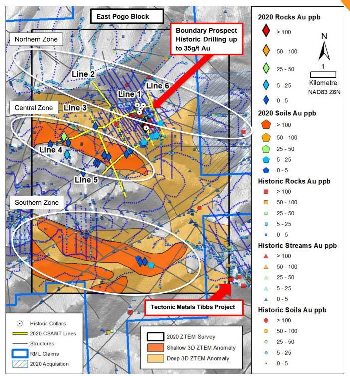
Figure 4 East Pogo Block: Historic and 2020 surface geochemistry indicating >95% of sampling reported <5ppb Au, supporting the Central Zone and Southern Zone being blind targets. Location of CSAMT survey lines, ZTEM survey area with footprint defined for geophysical anomalies. Note: Shallow CSAMT anomaly coincides with shallow ZTEM anomaly on the Central Zone.
